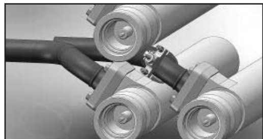
This computer image shows feeder pipes, in black, passing through a fuel channel, in grey. The FOLTM sensor is shown in the centre of the image and includes a custom-designed clamp with an integrated sensor around the pipe.
